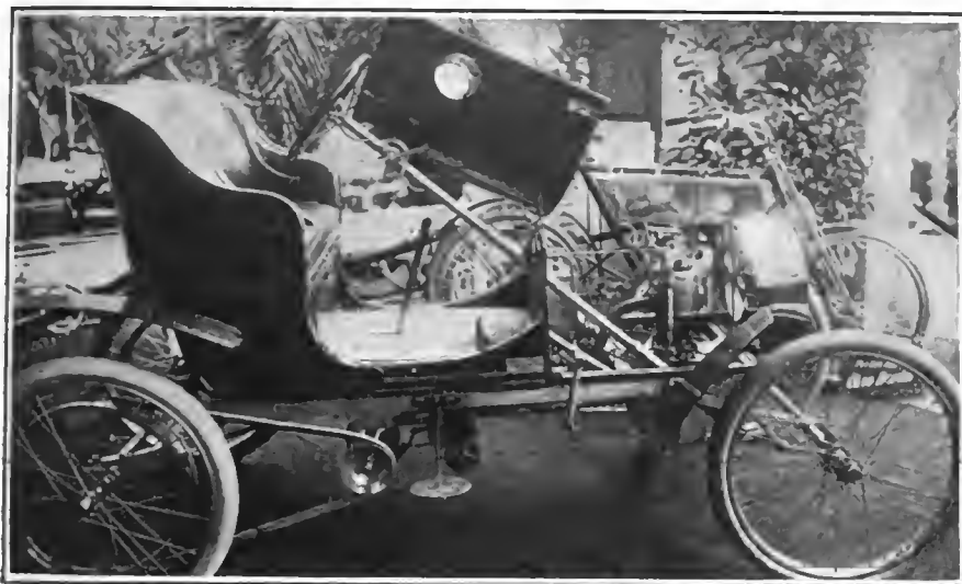
FIG. 3.—AIR-COOLED 5-HORSEPOWER OTAV SMALL ITALIAN CAR.
